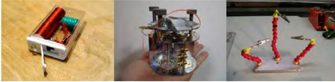
Figure 6: (from left to right) Inductive charge flashlight in candy bottle; atomic force microscope using DVD read head for probe control; a third hand tool from tripod.
