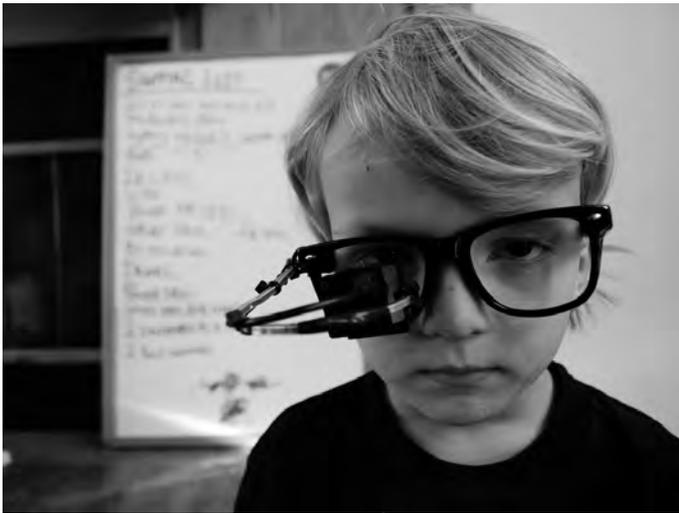
Figure 1: Example DIY project; an eye tracking system for the mobility impaired that costs two orders of magnitude less than commercial alternatives (The 'Eyewriter' [26]).
