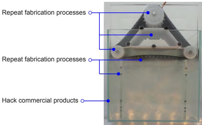
Figure 12: Development of a lid driven cavity flow chamber.
