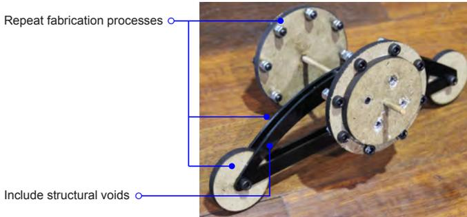
Figure 11: Sample prototype from experimental group; note the use of structural voids (hollow frame) and repeated manufacture (all custom parts were laser cut).
