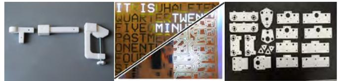
Figure 9: (from left to right) Clamp system for a modular MAV design where all custom parts are 3D printed; a light up clock, both the circuit and light stencil have been fabricated with the inkjet print and transfer PCB method; structural components for a CNC mill, all formed on laser cutter.
