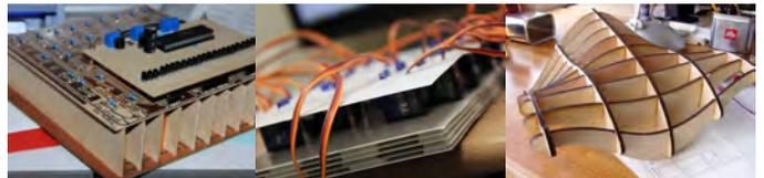
Figure 10: (from left to right) Light up display with polystyrene thin walls; servo actuated with paper case; laptop stand with bilaterally segmented laser-cut sheet assembly.
