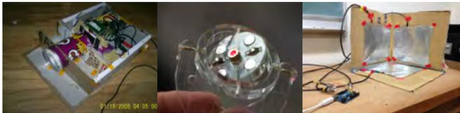
Figure 7: (from left to right) A projection system using cardboard, LEDs and a small LCD; a 3D magnetic field mapping tool using acrylic sheet, permanent magnets, and a handheld laser pointer; a 3D motion capture interface using an Arduino and three aluminum foil sheets.
