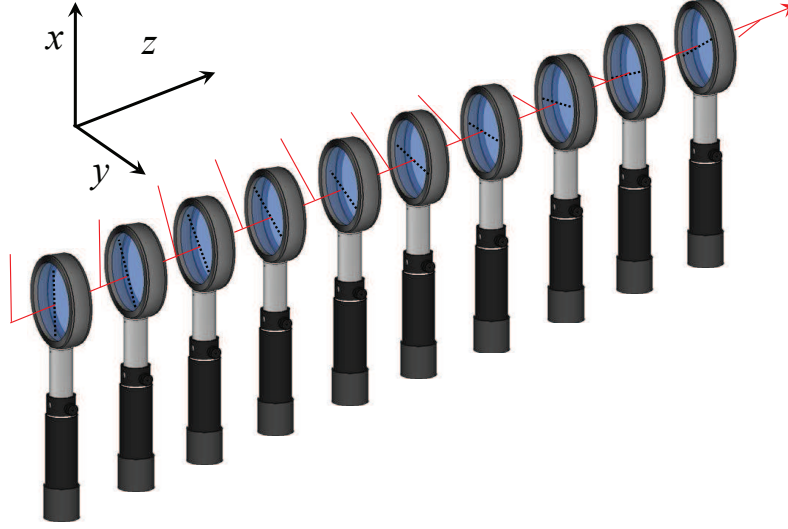
Figure 1. (Color online) Schematic illustration of a discrete adiabatic light evolution, which consists of a series of birefringent modules, separated by free-space propagation. The fast polarization axes of the wave plates are represented by dashed lines, while the solid red lines represent the orientation of linear polarization.
