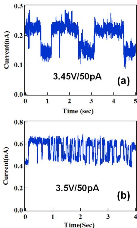
Figure 5. Observed RTN trends measured using an STM tip (with control current set at 50 pA) on a 5 nm  $\text{HfO}_2$  dielectric film at two different tip voltages of (a) 3.45V and (b) 3.50V [20]. Note that only a fraction of this voltage drops across the dielectric when we account for the finite voltage drop across the vacuum gap between the tip and film.
