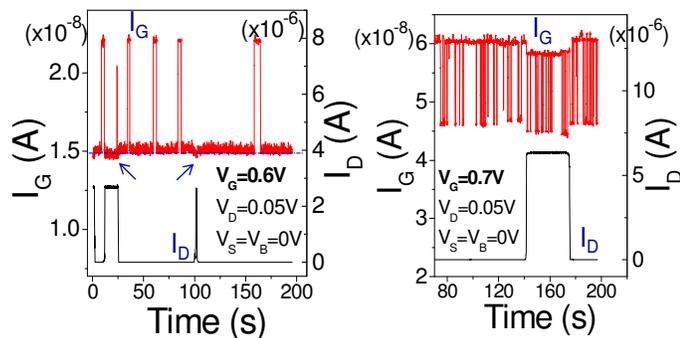
Figure 1. Observed  $I_g - I_d$  RTN trend at  $T = 150\text{K}$  showing one set of correlated signals and another set of uncorrelated signals embedded together, where these two signals correspond to two different defects in the dielectric (possibly located at very different locations from the Si-SiO<sub>x</sub> interface) [1].
