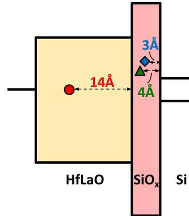
Figure 3. Band diagram showing the location of the three different defects responsible for the different  $I_g - I_d$  RTN patterns observed in Figs. 1 and 2 [1]. The defects situated deep in the high- $\kappa$  layer was the one which showed uncorrelated  $I_g - I_d$  trends (the  $I_d$  was not perturbed at all due to the minimal interaction with the discrete dopants situated far in the channel).
