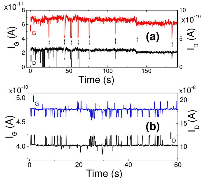
Figure 2. Observed  $I_g - I_d$  RTN trend at  $T = 77\text{K}$  showing (a)  $I_g \downarrow \rightarrow I_d \downarrow$  correlation measured at  $V_g/V_d = 0.5\text{V}/0.1\text{V}$  and (b)  $I_g \downarrow \rightarrow I_d \uparrow$  correlation measured at  $V_g/V_d = 0.6\text{V}/0.1\text{V}$ . Note that we are operating in the sub-threshold regime as  $V_{TH}$  was determined to be  $\sim 0.7\text{V}$  from post-SBD  $I_d - V_g$  measurements [1].
