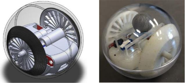
Figure 1. The design CAD model and prototype of VIRGO [6], a spherical robot (Diameter = 8 cm) under development at SUTD.
