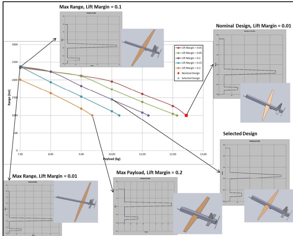
**Fig 3. Effect on design configurations on the Pareto curves by varying margins**
