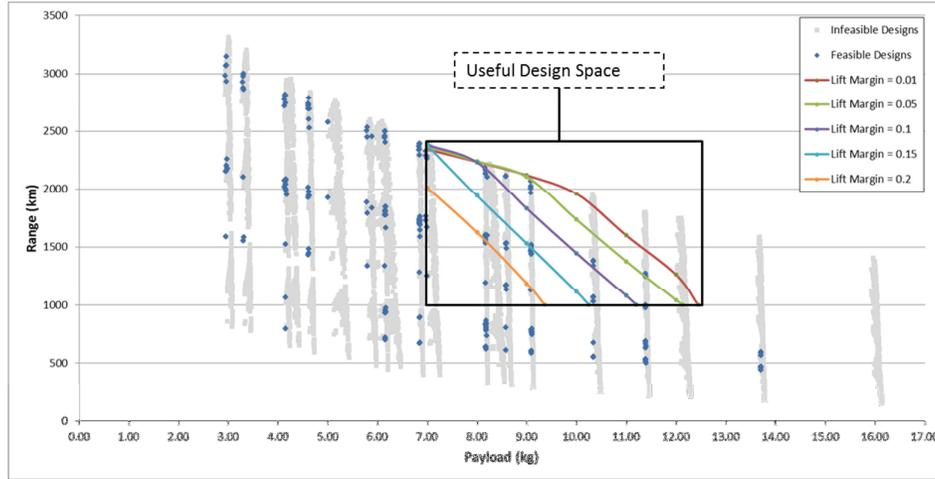
**Fig 1. Location of useful design space with relation to the Iso-margin curves**
