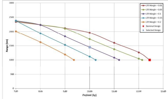
**Fig 2. Effect of varying margins on Pareto Range-Payload Performance**
