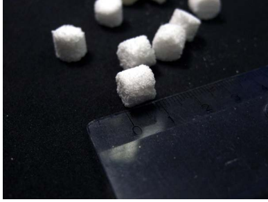
Figure 6. A sample of a piece of ceramic foam with h = 10 mm and r = 5 mm
