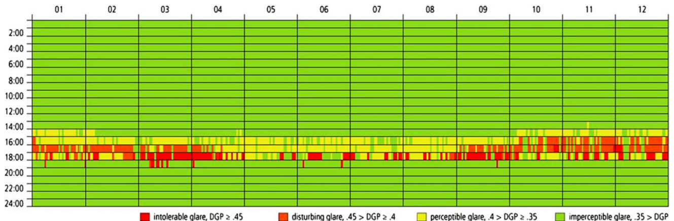
Fig. 2. Glare values over 1 year for a room of the church in Singapore, according to the date and time of day.
