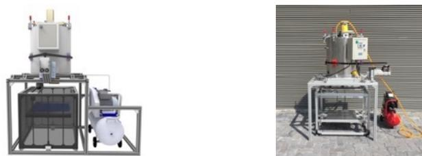
Figure 16: Integrated multi-phase engine printer. (left) Final system CAD. (right) Final system physical construction.
